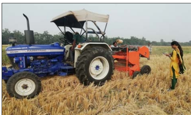
Fig 7: Field performance of tractor drawn round straw baler
