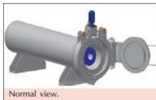
Fig 1: Supercritical instrument used for dyeing (Normal view)
