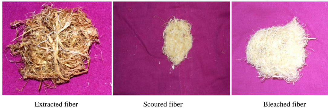
Fig 5: Corn stalk fibre a) Extracted, b) Scoured, c) Bleached
