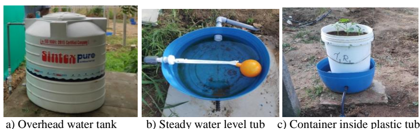
Fig 2: Components of matric suction irrigation assembly
