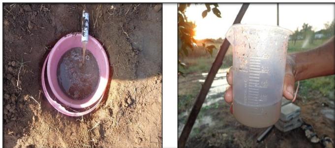
Fig 4: Measurement of runoff through volumetric method
