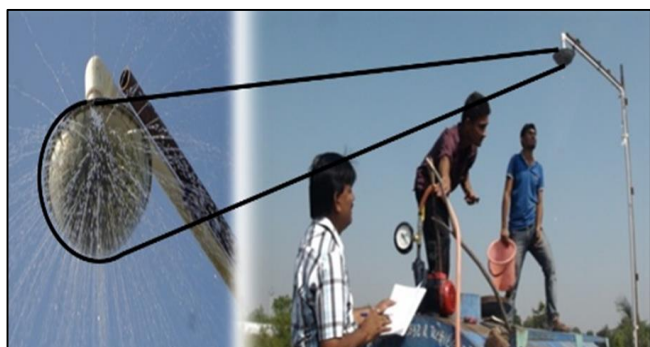
Fig 5: Calibration of input rainfall intensities during simulation
