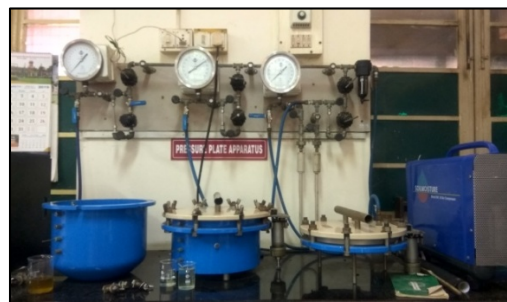
Fig 1: Determination of water holding capacity of the initial pot soil using pressure plate apparatus
