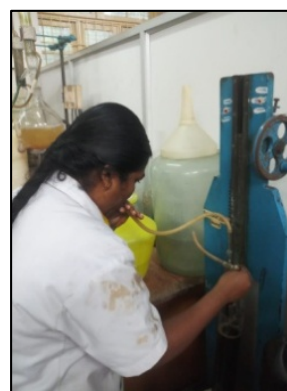
Fig 2: Determination of soil texture of the initial pot soil by International Robinson Pipette method
