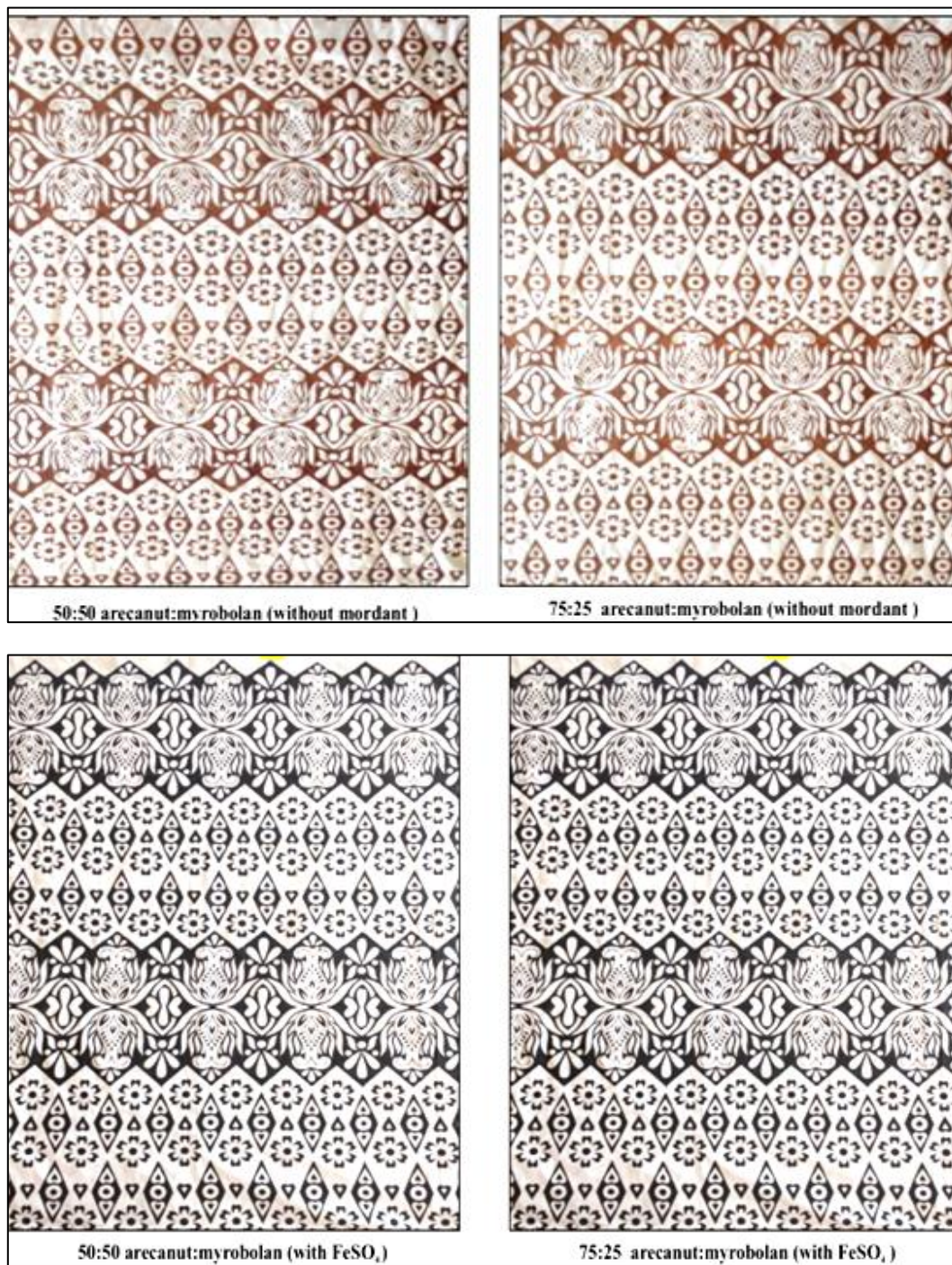
Plate 2: Samples printed with Arecanut: myrobolan pigment using sodium alginate gum (0.5%) with and without mordant
