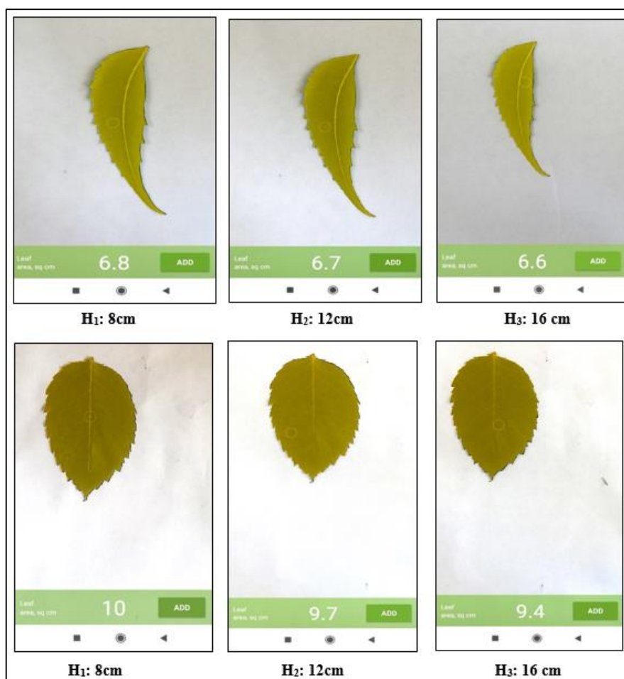
Fig 4: Effect of calibration height on the accuracy of the mobile application for the same leaf of both Neem and Rose
