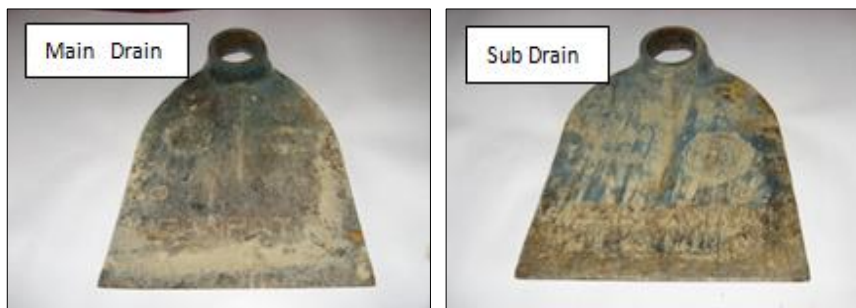
Fig 7: Improved blades for digging main drain and sub drain
