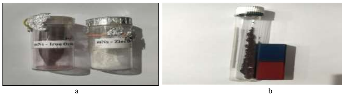
Fig 1: a. Readied nanocomposite b. Magnetic property of iron oxide in mNs.
