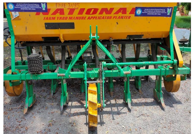
Fig 2: Tractor drawn FYM applicator cum seed drill
