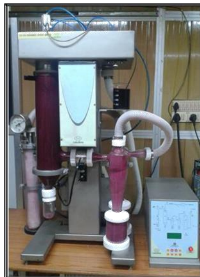
Plate 1: Lab scale twin cyclone spray dryer Labultima LU-222
