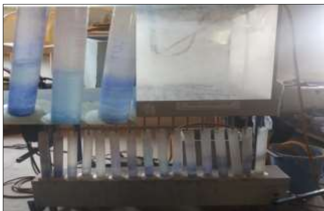
Fig 4: Spray liquid from the channels collected in the measuring jars
