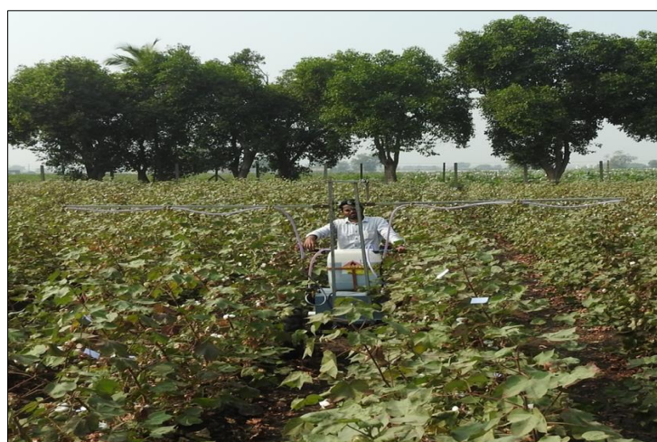
Fig 7: Nozzle adjustment from the plant canopy
