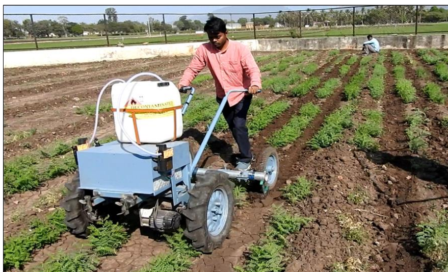
Fig 5: Snapshot of the developed machine with weeding attachment
