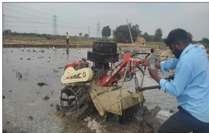
Plate 4: Noise measurements at operators ears position
