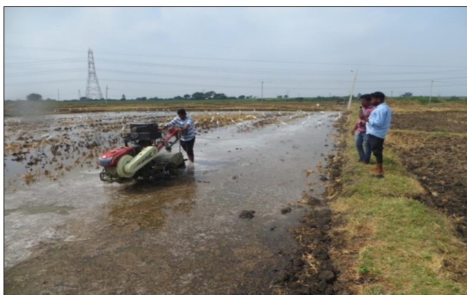
Plate 3: Noise measurements at by standers position of power tiller
