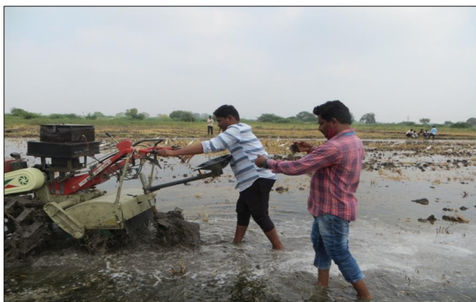
Plate 2: Vibration measurements at handle of power tiller during field operation
