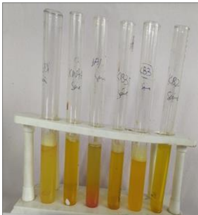
Plate 8: The change in color to brown, to red or dark yellow shows a positive ammonia production test
