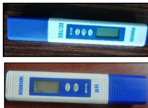
Fig 4: Aquasol Pen type EC/TDS and pH meter used in the experiment
