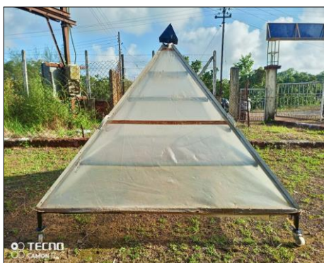
Plate 1: Pyramid shape foldable solar dryer
