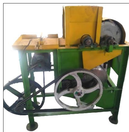
Fig 4: Developed power operated raw mango cutting machine
