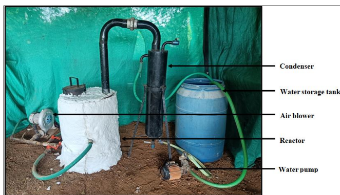
Fig 2: Pictorial view of complete pyrolysis set-up
