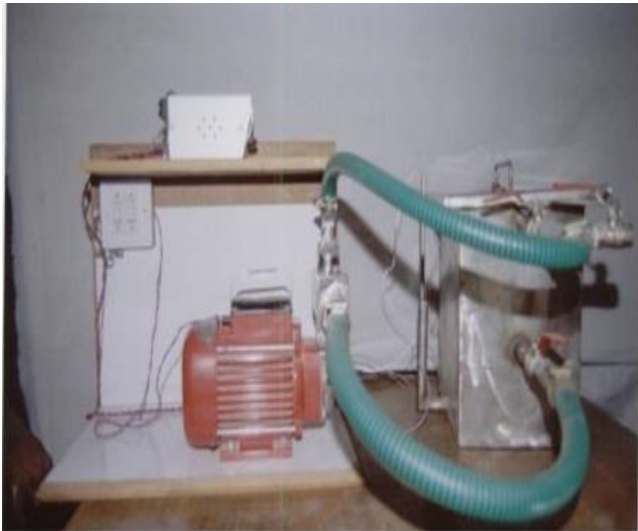
Fig 2: Schematic diagram of osmotic dehydration unit
