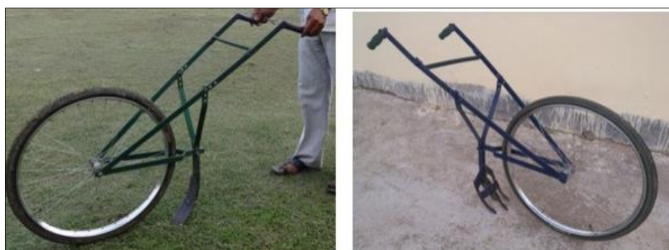
Fig 12: (A) Push and pull type cycle weeder (B) Modified Push and pull type cycle weeder.
