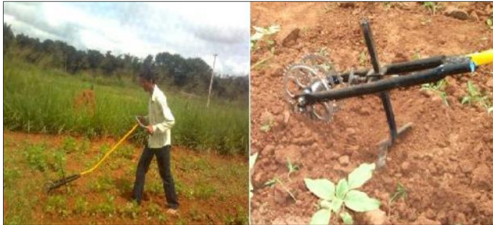
Fig 6: The weeding operation by sprocket weeder
