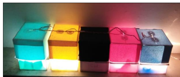
Fig 1: Growth chambers equipped with (a) green (b) yellow (c) no light (d) red (e) blue
