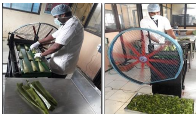
Plate 1: Performance evaluation of Aloe vera leaf slicing machine
