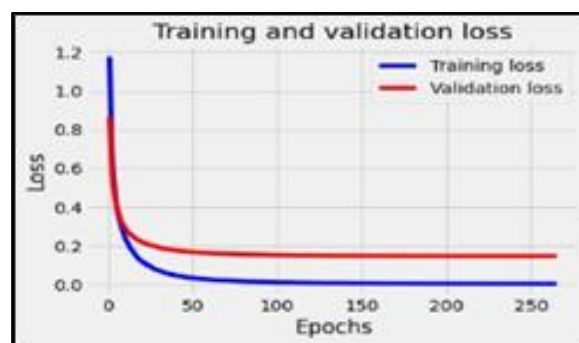
Fig 7: Train & validation loss of VGG16 at batch size 128
