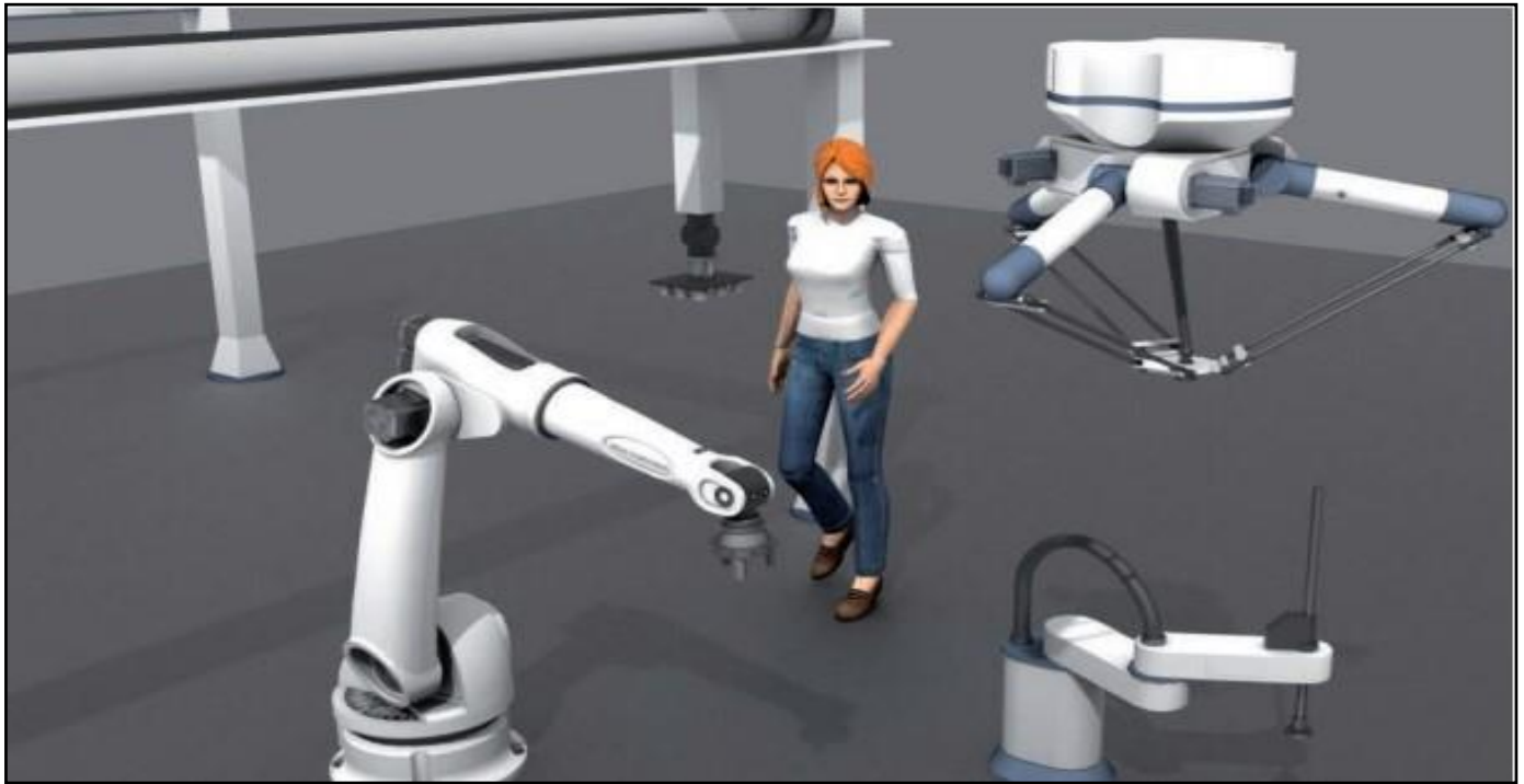
Fig 2.1: Types of robot with respect to kinematics
