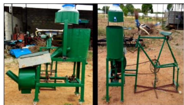
Fig 1: Fabrication of pedal operated integrated potato peeler and slicer (a) front view, (b) side view
