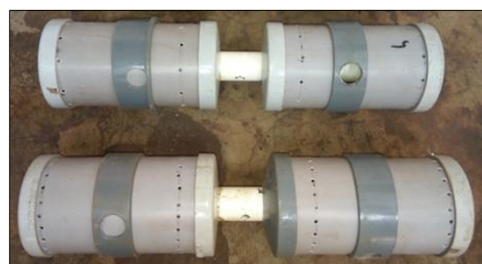
Fig 2: Seed metering drums fitted on PVC pipe
