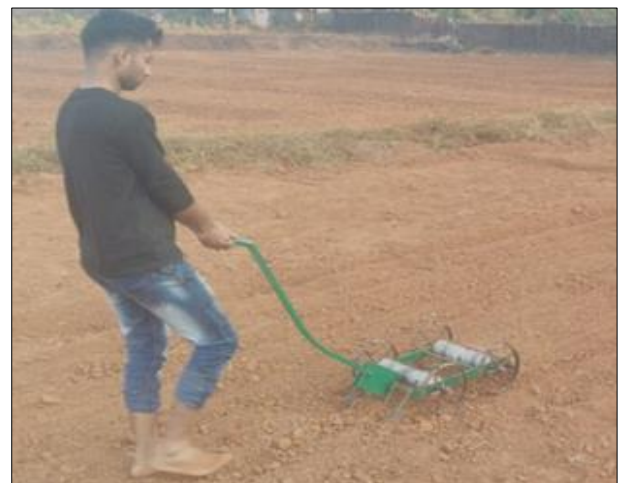
Fig 8: Developed manually operated seed cum fertilizer drum seeder for finger millet for nursery raising in operation
