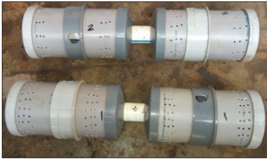
Fig 3: Fertilizer metering drums fitted on PVC pipe
