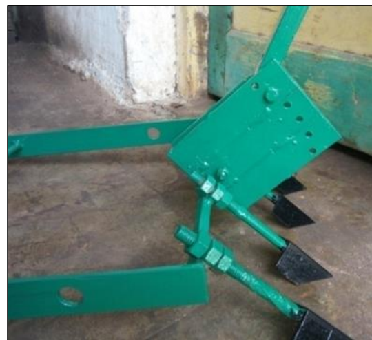
Fig 7: Arrangement for changing the angle of the handle in vertical plane
