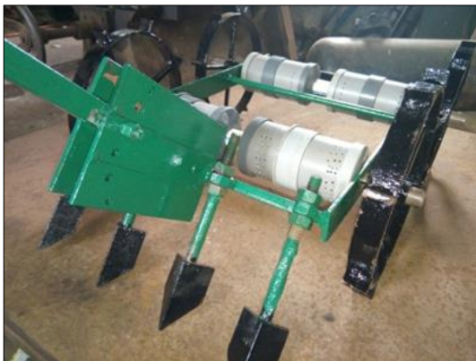
Fig 4: Seed and fertilizer drums mounted on the main frame
