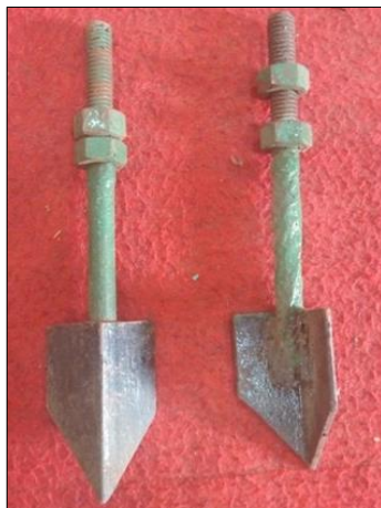
Fig 5: Furrow openers of the manually operated seed cum fertilizer drum seeder for finger millet
