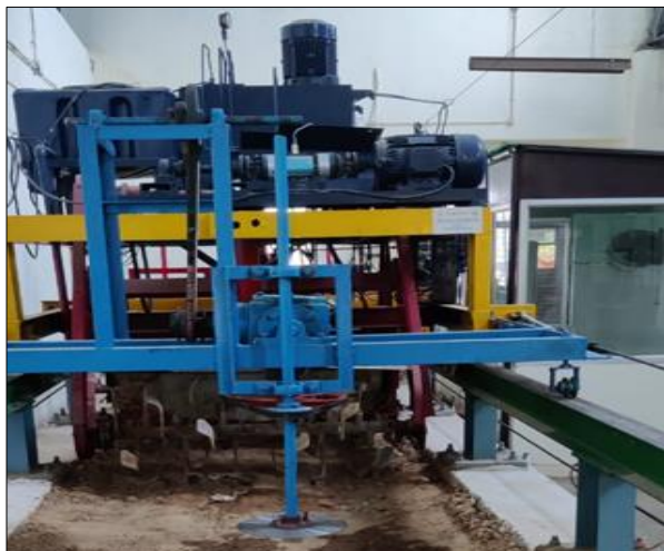
(a) Test trolley, processing trolley and vertical rotor
