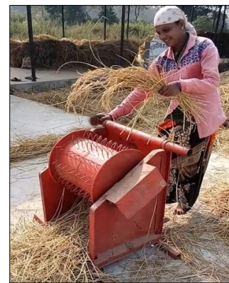
Fig 3: Tribal women during operation of pedal operated thresher with paddy
