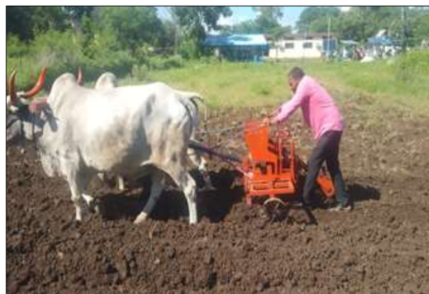
Fig 3: Turmeric planting with Developed turmeric planter
