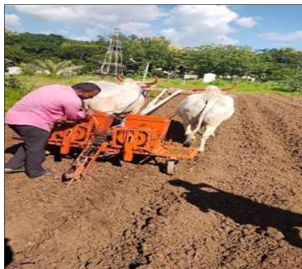
Fig 1: Turmeric planting with developed bullock drawn turmeric planter
