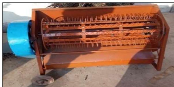
Fig 3: Motor operated paddy thresher
