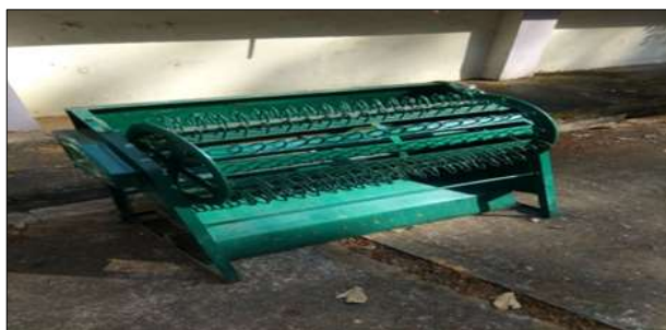
Fig 2: Foot operated paddy thresher
