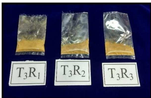
Plate 3: Aloe vera pulp powder prepared from sample dried by microwave drying method
