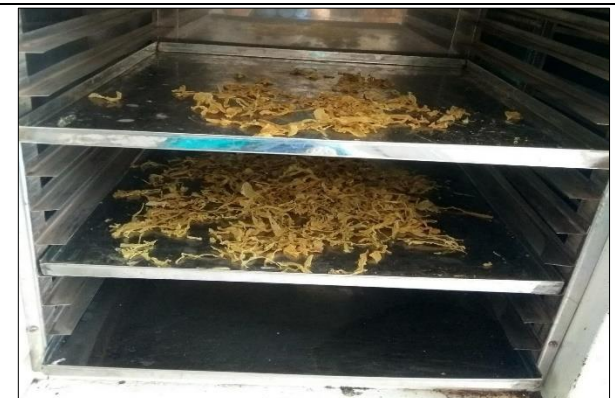
Plate 8: Convective dried sample of fresh Aloe vera pulp fillets
