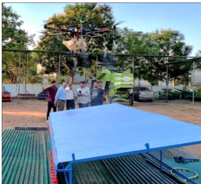
Fig 4: Stabilization of the drone over Patternater
