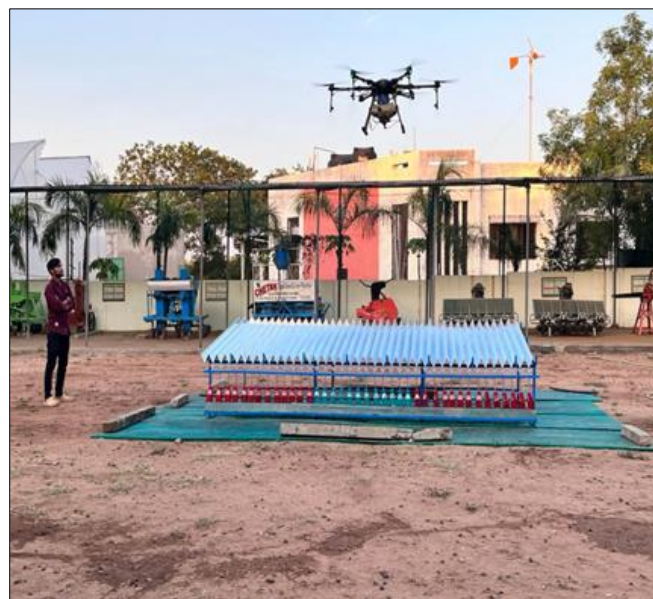
Fig 5: Spraying of liquid by drone on the patternater
