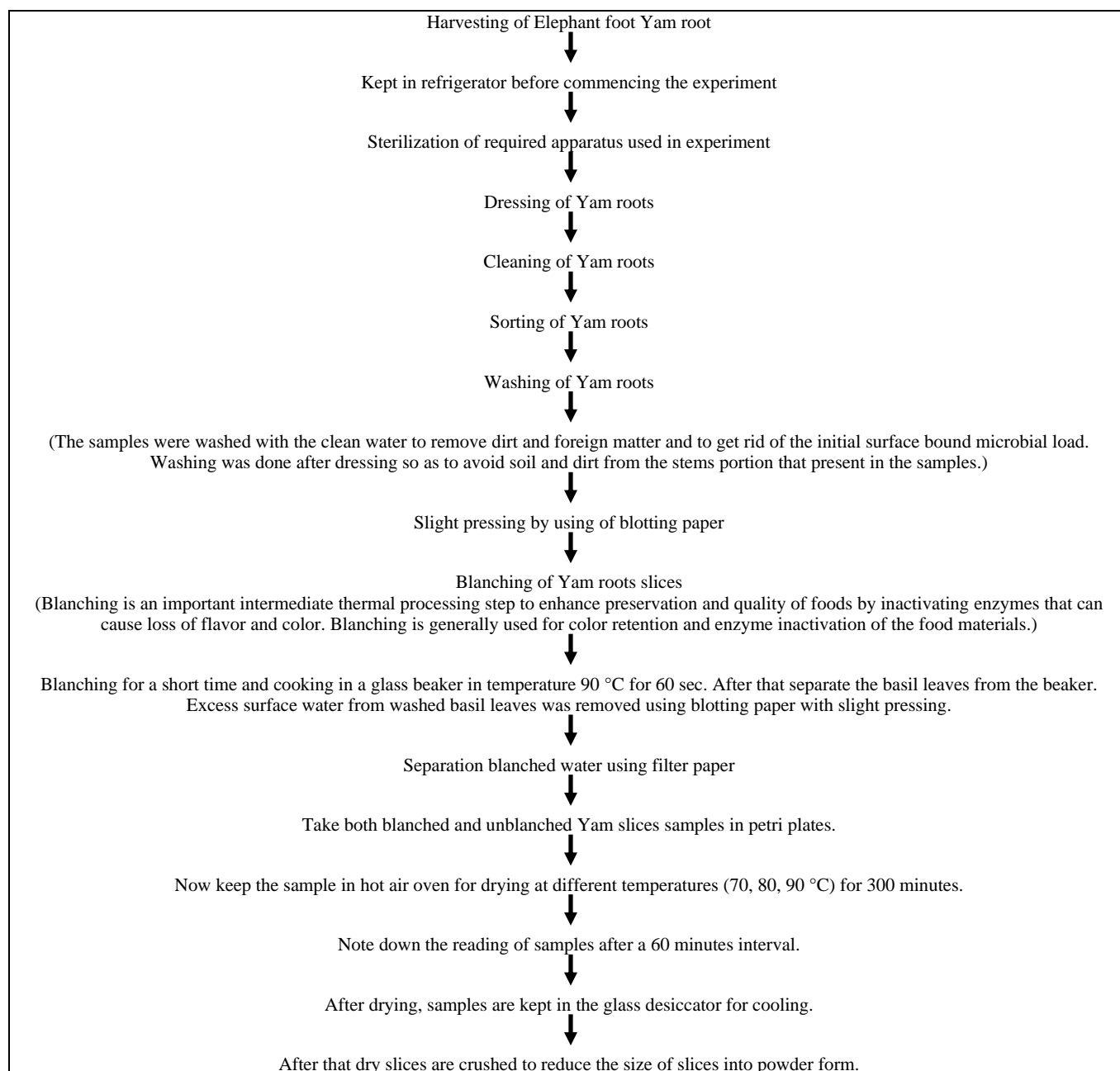
Fig 4: Flow chart of processing Yam powder
