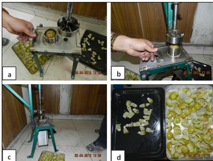
Fig 4: Operation of the machine: a & b feeding of fruit, c- punching and cutting, d- fruit segments and seeds
