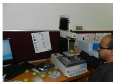
Shear test with blade set
