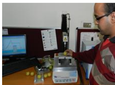
Puncture test with needle probe
