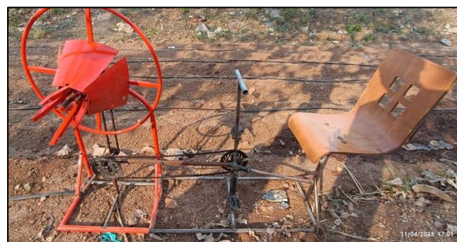
Plate 8: Pedal operated drip lateral winder
