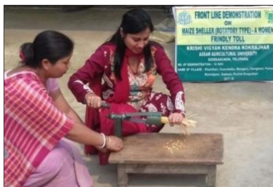
Women shelling grains from maize cob with rotatory hand maize sheller
