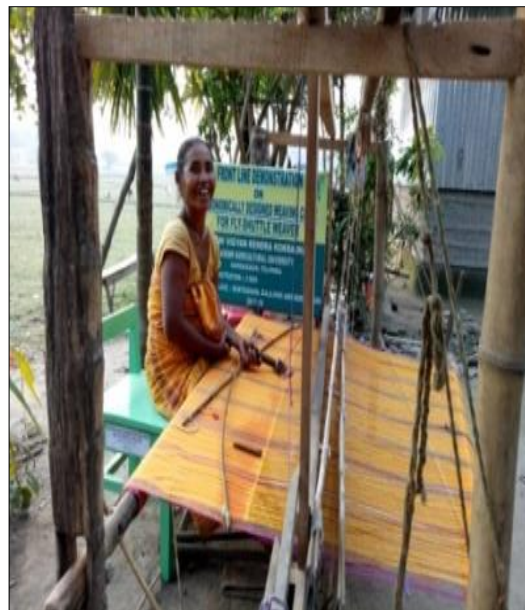
Women weaves in Fly shuttle loom and sit comfortably in ergonomically designed weaving chair
