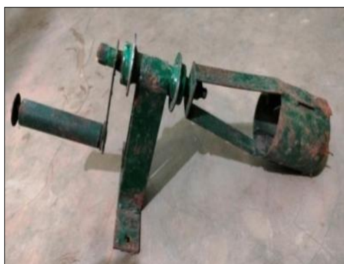
Fig 3: Maize sheller (Rotatory type)
