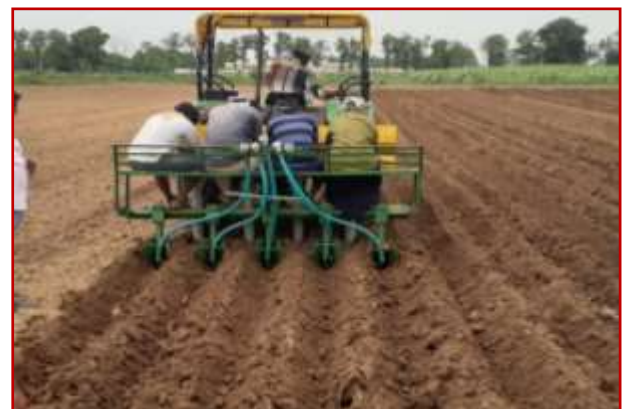
Fig 2: Sowing operation of turmeric with 4-row seed drill (ridge and furrow method)
