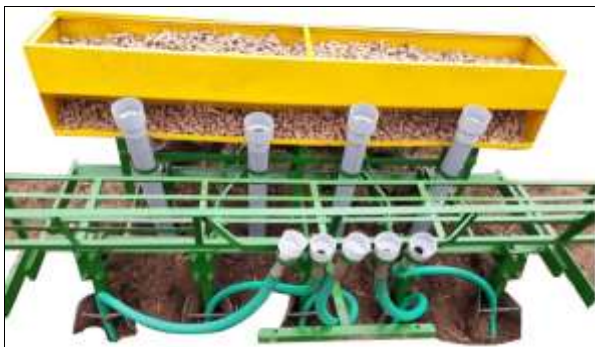
Fig 1: View of 4-row turmeric seed drill.
