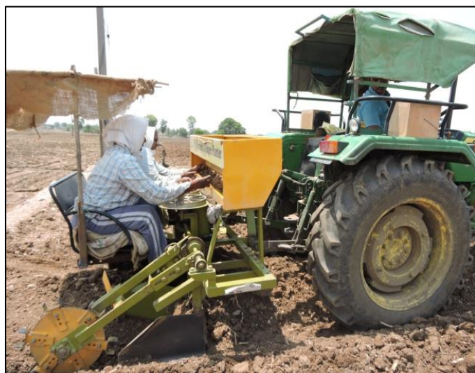
Fig 1: View of 2-row raised bed turmeric semi-automatic planter.
