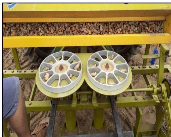
Fig 2: Sowing operation of 2-row raised bed turmeric semi-automatic planter
