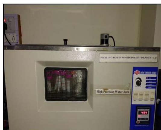
Plate 1: Enzymatic hydrolysis of samples loaded with CTec2 Cellulase enzyme in water bath incubator shaker
