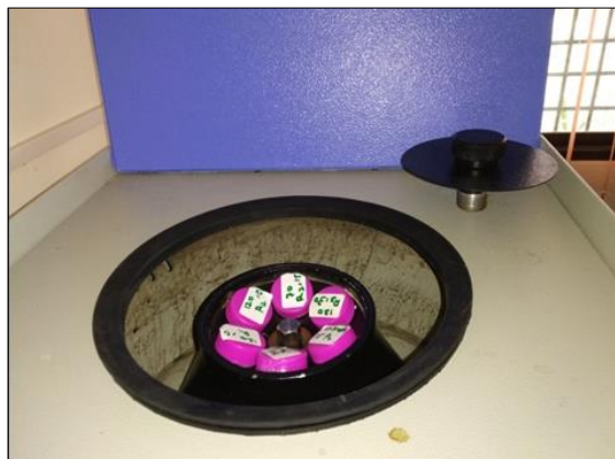
Plate 2: Enzymatic hydrolyzed samples kept for centrifugation in high speed refrigerated centrifuge
