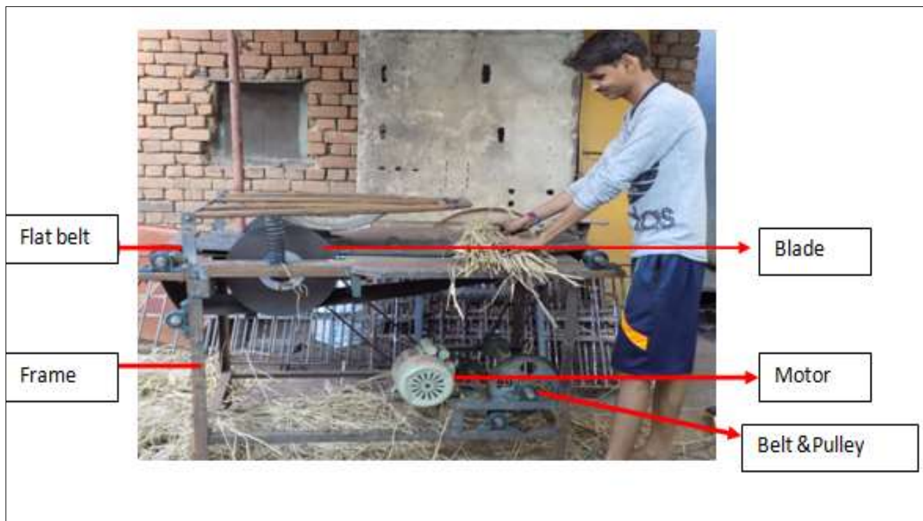
Fig 1: Developed power operated paddy straw size cutter
