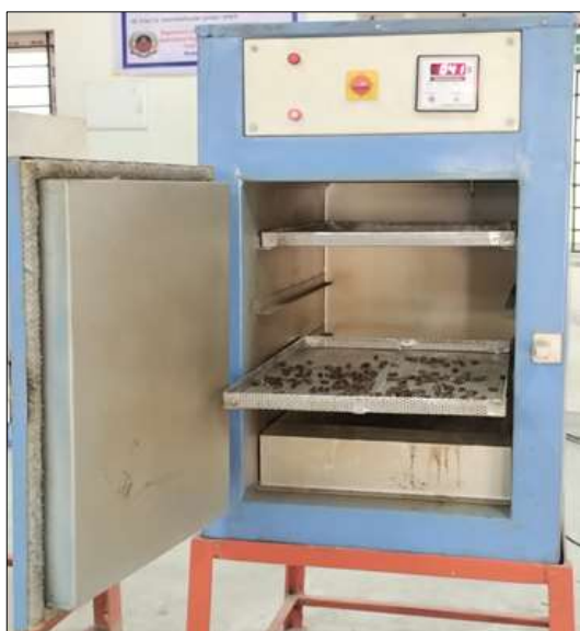
Fig 2: Measurement of moisture content of neem fruits using hot air oven
