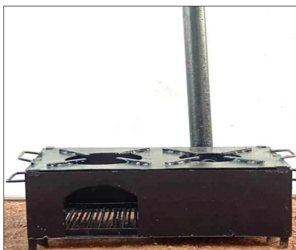
Developed integrated cook stove and barbeque unit
