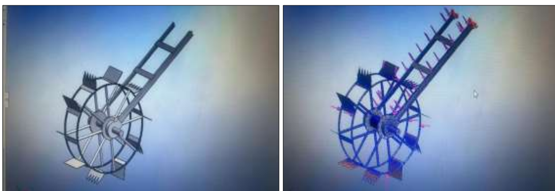
Fig 2: 3-D model of weeder frame with mesh generation
