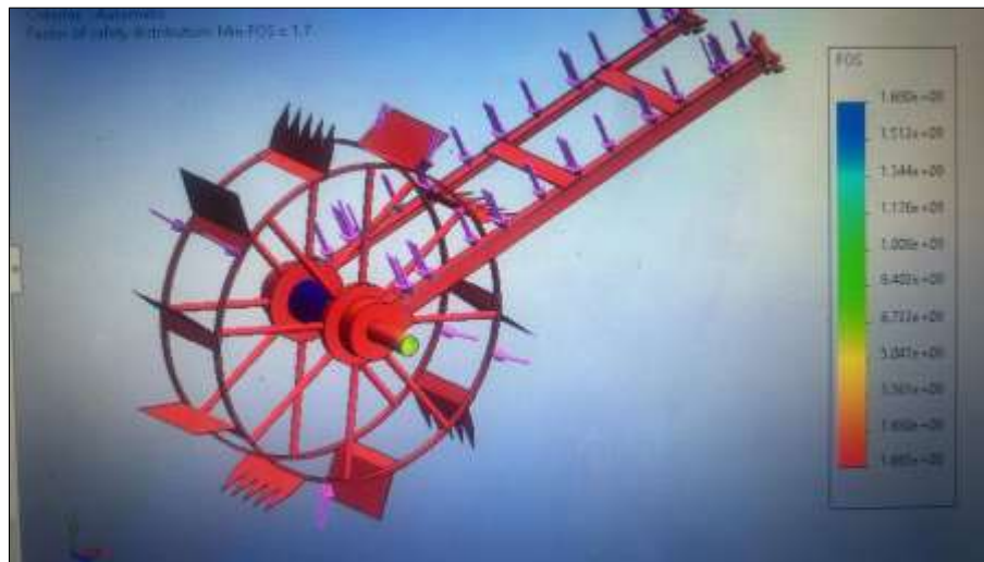
Fig 5: Factor of safety diagram of finite element analysis
