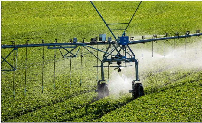
Fig 4: VRI installed in centre pivot system of irrigation (source: valleyirrigation.com)
