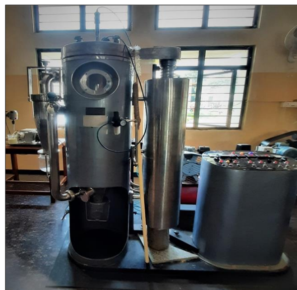
Fig 3: Tall type spray drier
