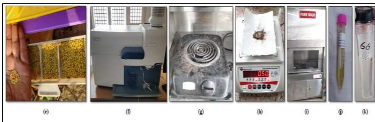
Fig 1: (a) Soil sample (b) Pollen sample (c) Collection of fresh nectar and honey from bee hive frames (d) Honey sampling (e) Collection of pollen with the help of pollen traps (f) Heavy metals detection by using microwave plasma atomic emission spectroscopy (MP-AES 4200) (g) Hot plate used for heating the samples (h) Electronic balance used for weighing samples (i) Fume hood used for sample digestion (j) Nectar sample (k) Sample digestion in culture tube.
