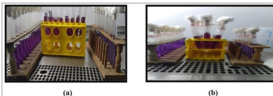
Plate 1: Water samples containing MacConkey lactose bile broth with Durham's tubes before incubation
